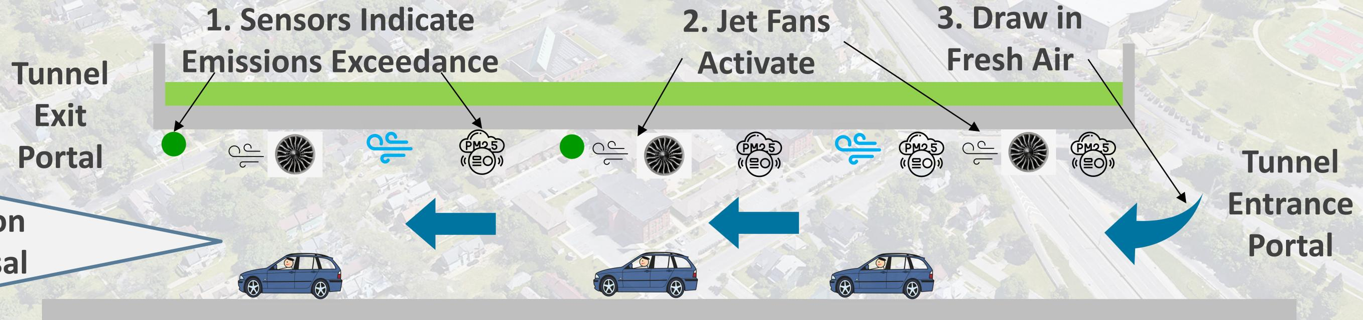
Longitudinal Profile of Tunnel
